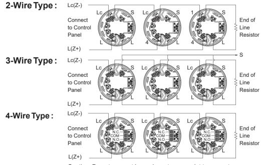
Caution: Do not connect loop wires at same point to prevent function loss.
