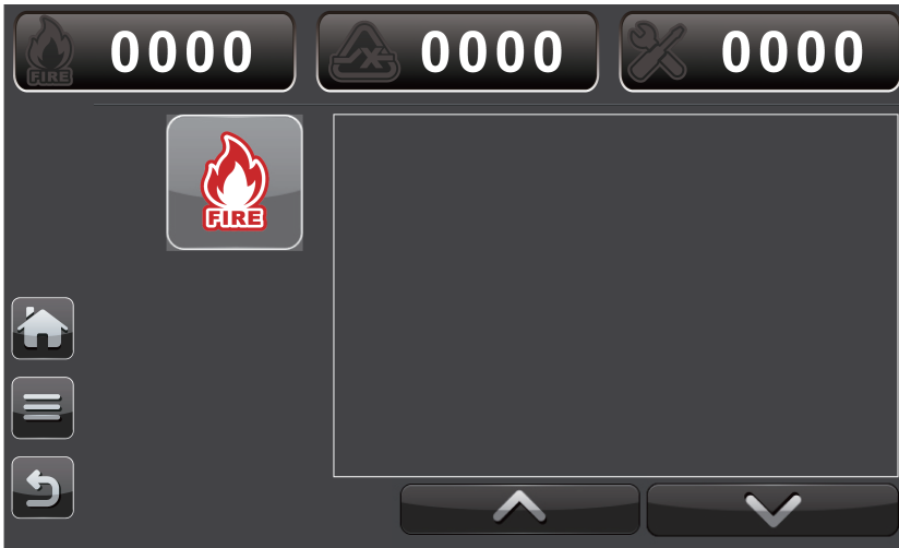
【 Figure 1: No fire Alarm event on LCD screen 】
