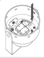
Fuel the CLEANING NAPHTHA into the fuel cup (≦40cc),make the cotton fully absorbed.
